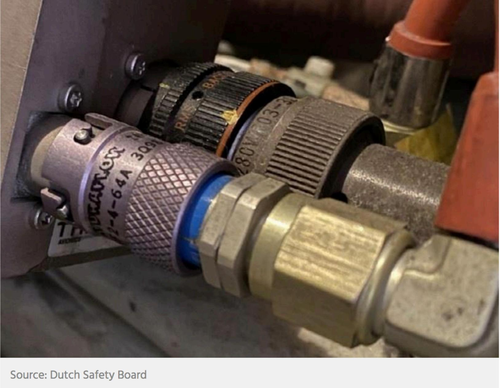
Quick-disconnect fittings were not attached to the air-data modules
