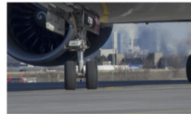
Source: Air Canada Investigators heard the 777-300ER nose gear had a lamp signaling parking brake activation
