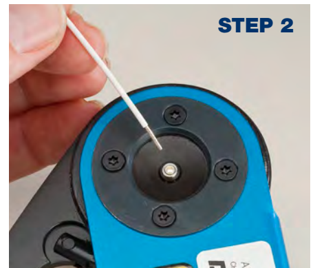
INSERT PRE-STRIPPED WIRE
