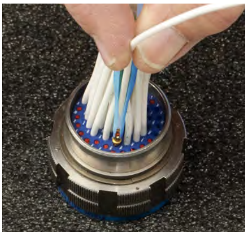
Typical All Plastic Tool Operation
