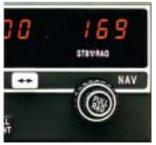
IDENT: The NAV "IDENT" knob is activated by pulling it outward, so that both voice and ident can be heard. When this knob is pushed in, the ident tone is muted. Volume of voice/ident can be adjusted by turning this knob—clockwise to increase, counterclockwise to decrease.
