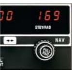
The lower-cost KX 155 system is virtually identical in appearance to the KX 165; however, it doesn't include the digital Radial readout feature. Also, the KX 155 requires an external VOR/LOC converter (usually included n the appropriate Bendix/King NAV indicator) while the KX 165 comes with a built-in VOR/LOC converter designed to interface directly with any ARINC standard CDI or HSI display.
