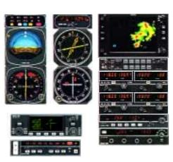
A complete package for the sophisticated panel. The KX 165 is both the number one and number two NAV/COMM in this configuration. Long-range navigation is provided by the KLN 90B GPS, and Mode S transponder capability is offered by the KT 70. Full IFR performance and a KFC 150 Flight Director/Autopilot make this the most complete avionics package available from one manufacturer.
