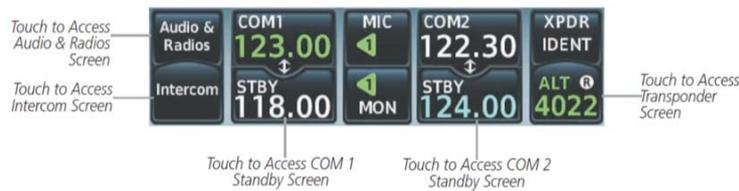
The Label Bar, near the bottom of the Touchscreen Controller and above the **Joystick** and **Knobs** displays the current function of each physical control on the Touchscreen Controller as a reference. These functions include Map Range adjustment, display pane selection, radio volume/squelch adjustment, COM radio tuning, and alphanumeric data entry.
