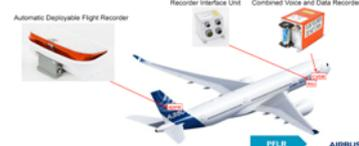
Automatic Deployable Flight Recorder, Recorder Interface Unit, Combined Voice and Data Recorder
