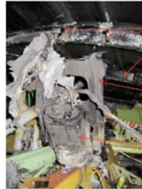
Figure 9 ELT and ELT mounting plate, view on forward end, looking aft
